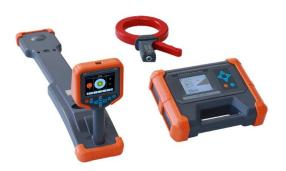
GD-3134E is a set of high-performance special underground cable path detection and identification instrument, which is composed of signal transmitter and receiver. It can be used for path detection, depth measurement and pipeline survey of underground cables and metal pipelines. With a variety of optional accessories, it can carry out unique identification and find pipeline insulation damage and some types of cable faults.
